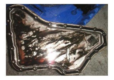
^ dirty oil or oil that has surpassed its temperature limits, this would indicate friction component (band or clutch disc) breakdown and in order to be sure all of the debris is out of the <a href="ATF">ATF</a> cooling system, complete replacement of the ATF cooling system (radiator, auxiliary cooler [if applicable], and cooler lines) is required. See photo.
