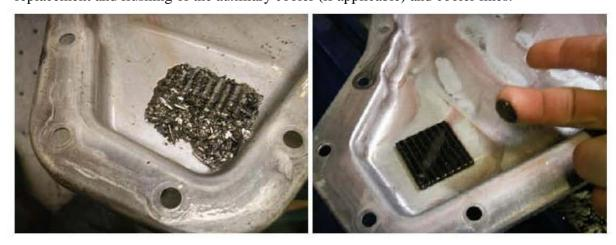
^ metal in the transmission fluid, this would indicate an internal transmission problem. **Note!** Metal in the <u>ATF</u> is nearly impossible to flush out completely. In order to be rid of all metal particles, complete replacement of the ATF cooling system (radiator, auxiliary cooler [if applicable], and cooler lines) is required. See photo. Black sediment on the pan magnet is normal. See photo.
